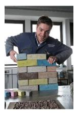
A group of engineers from the <u>Heriot-Watt University in Scotland</u> started a company called **Kenoteq**, which designed an environmentally friendly brick. This new brick is called the **K-Briq**, and 90% of it is made with construction waste. Furthermore, its production doesn't require a kiln, and generates only one tenth the carbon emissions of conventional bricks.
